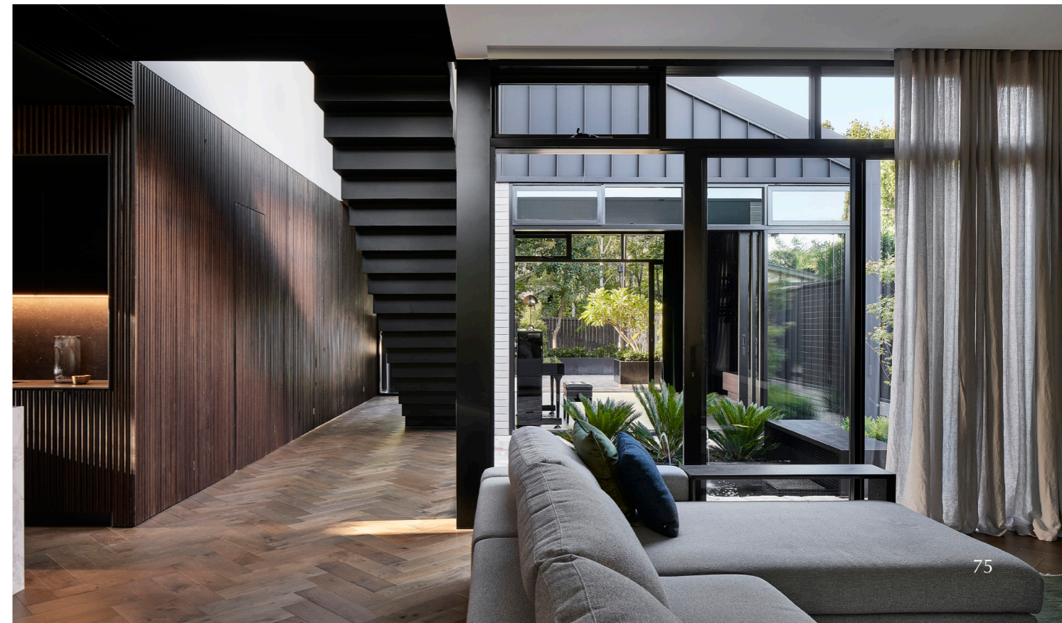
The steel staircase (below) was prefabricated off site and craned into position. Dark finishes and touches of metallics throughout the house (above and left) add contemporary sophistication.
